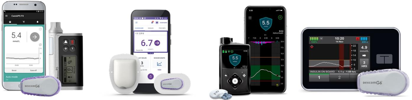
A hybrid closed loop (HCL) is a system which involves one of the pumps working together with one of the CGMs.
